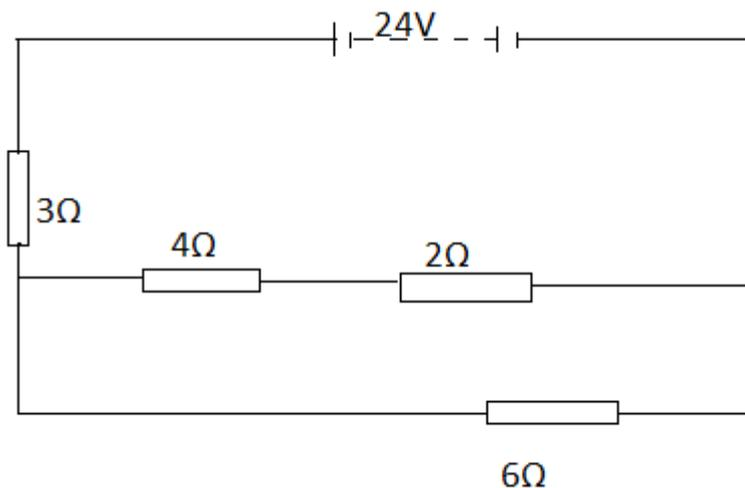
An accumulator of e.m.f. 24V and internal resistance of  $2\Omega$ , is connected to  $3\Omega$ ,  $4\Omega$ ,  $2\Omega$ , and  $6\Omega$  resistors as shown in the diagram above.
