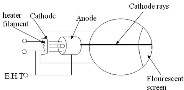
When a cathode is heated, electrons are emitted by thermionic emission process. The emitted electrons are accelerated by
