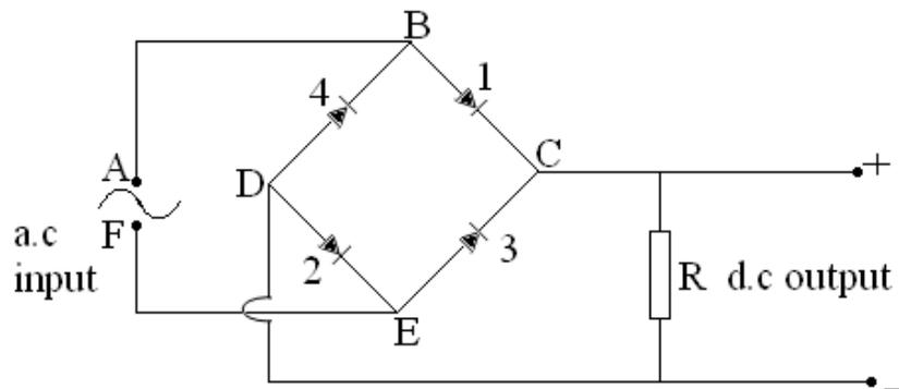
If A is positive during the first half-cycle, diodes 1 and 2 conduct current along ABC through R and back through DEF.
