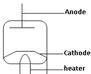
The valve is made up of two electrodes; the anode, the cathode which is heated up by a heater connected to a low voltage supply.
