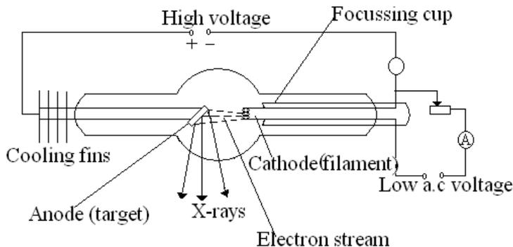
Electrons from a hot filament are produced by thermionic emission. The electrons are accelerated by the high potential difference
