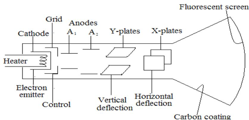
The chief feature of an oscilloscope is the cathode ray tube, which is a vacuum tube containing three major components:
