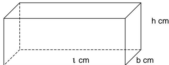
$$\text{Volume} = \text{length} \times \text{breadth} \times \text{height}$$
