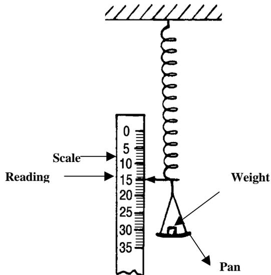
The force is due to the weight placed in the pan. Typical results are as follows:
