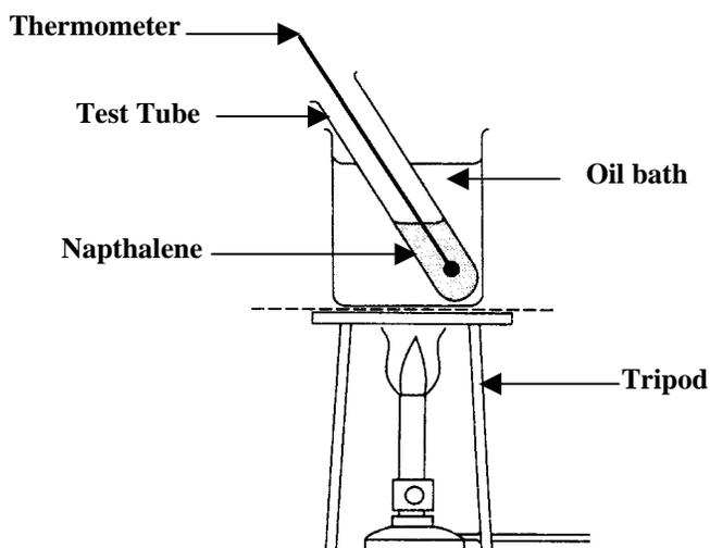
Heat the liquid i.e. the oil and stir with the glass rod. Observe carefully. When the solid naphthalene melts, stop heating. Record the temperature. This is the melting point of naphthalene.
