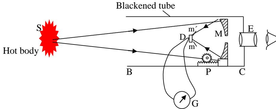
It consists of a blackened tube, open at end B. D is a thermocouple attached to a small blackened copper disc facing end C and is shielded from direct radiation. M is a gold-plated mirror, pierced at its centre to allow radiation to reach the eyepiece, and movable by a rack and pinion P.
