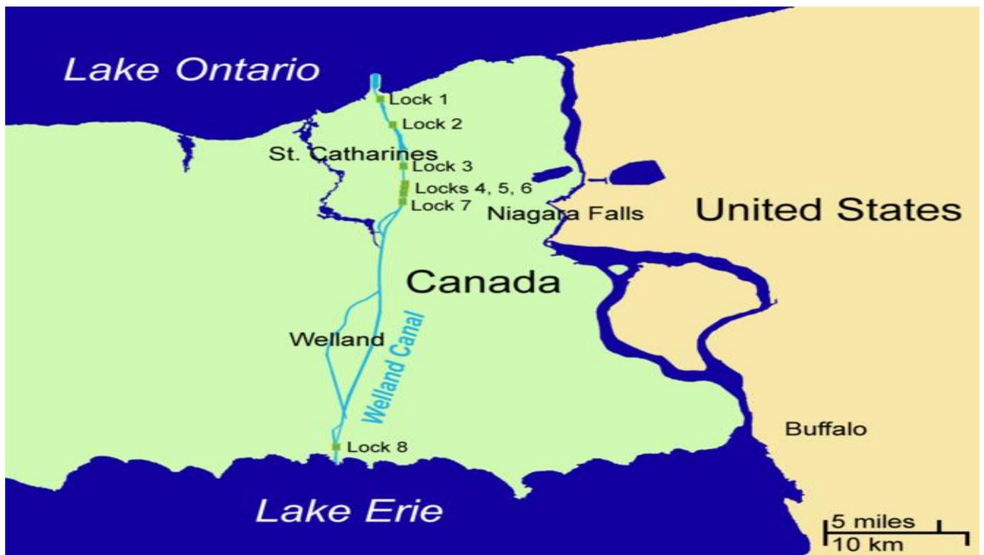
The original canal was built in the 1860's and improvements were made several times until 1932 when a modern ship canal was constructed. There are eight (8) locks on the Welland canal. As part of the Saint Lawrence sea way project, further improvements were made on the Welland canal and these included the following:
