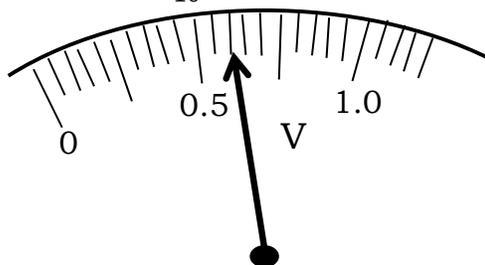
The illustration above shows a voltmeter reading =  $(12 \times 0.05) = 0.60$  V.
