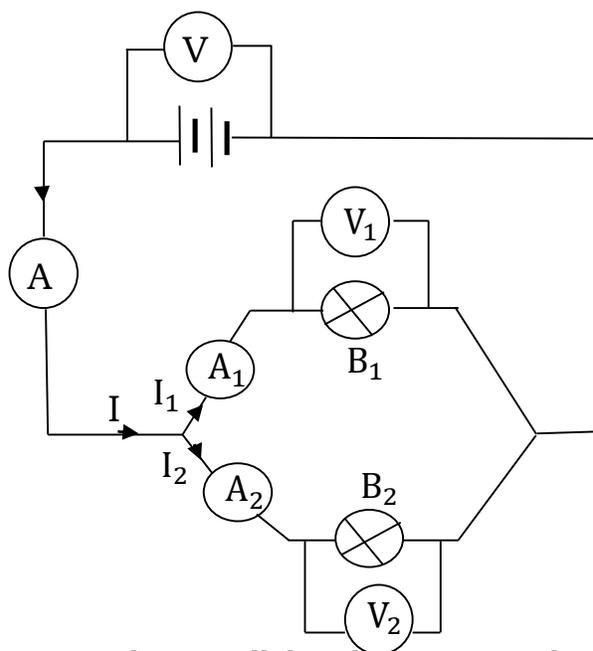
Bulbs  $B_1$  and  $B_2$  are connected in parallel in the circuit as shown above.
