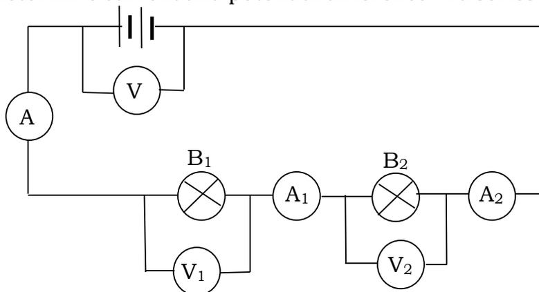
Bulbs B<sub>1</sub> and B<sub>2</sub> are connected in the circuit as shown above.
