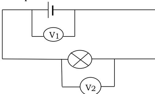
Voltmeter  $V_1$  measures the p.d between the terminals of the cell, while  $V_2$  measures the p.d across the bulb.
