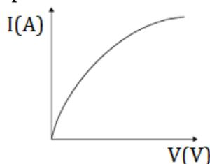
The graph is non-linear (not a straight line). This means that current is not directly proportional to the potential difference in a filament lamp because the temperature does not remain constant.
