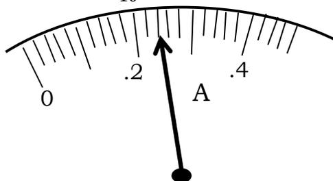
The illustration above shows an ammeter reading =  $(12 \times 0.02) = 0.24$  A.
