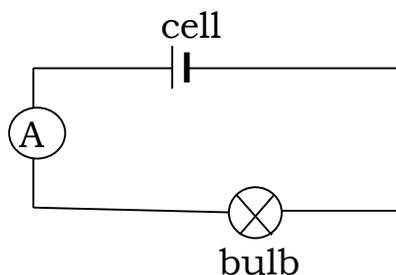
This ensures that the current that passes through the device is the same current that passes through the ammeter.
