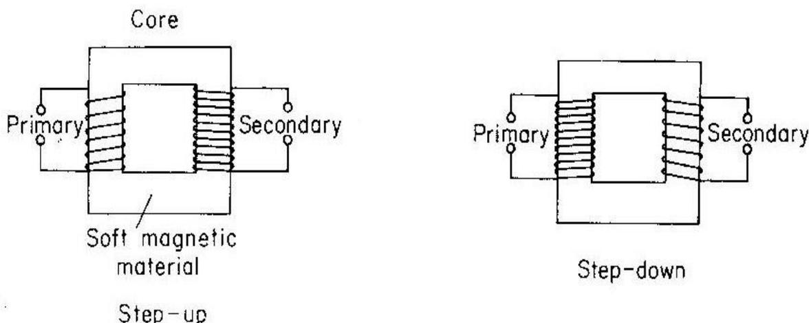
When an alternating p.d is applied to the primary coil, the resultant current produces a large alternating magnetic flux which links with the secondary coil and induces an e.m.f in it.
