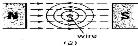
The field due to current carrying wire is indicated by the circles while the dotted lines are field lines of magnet.
