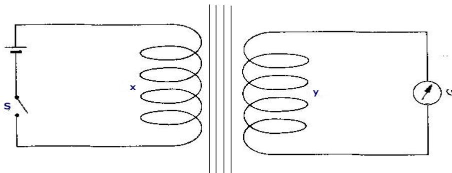
When the switch is closed, electric current flows through the primary coil. As the current builds up in the coil from zero to its maximum value, it sets up a varying magnetic field around it that induces an e.m.f. in the neighboring coil.
