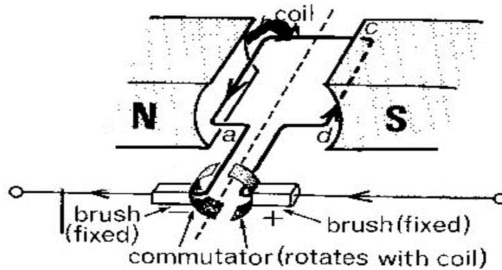
The Simple d.c motor consists of a rectangular coil of wire placed between pieces of a strong magnet, and its ends are connected to half – split commutators. The commutators are each in contact with a carbon brush which are in turn connected to a d.c supply. The coil is free to rotate in the uniform magnetic field.
