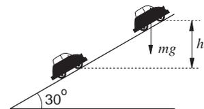
For a car of mass  $m$  the work done against gravity is still  $mgh$ . Since this result does not involve the angle of the slope,  $\theta$ , it is the same for **any** slope.
