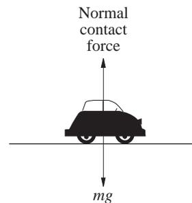
The distance the car moves in the direction of either of these forces is zero and so these forces do no work.
