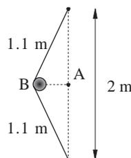
The rock B of mass 20 kg is in the catapult as shown. Calculate the speed with which the rock is released at A when the elastic string returns to its natural length of 2 m if the string's stiffness is  $250 \text{ Nm}^{-1}$
