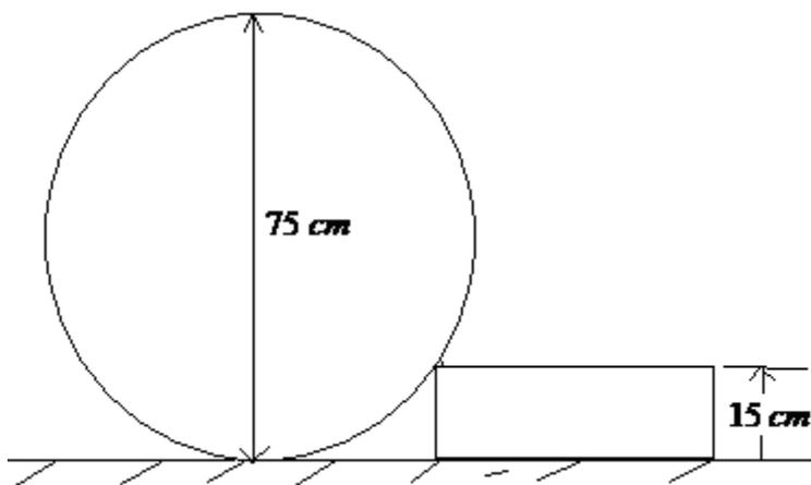
Find the least horizontal force applied through the centre of the drum, which will cause the drum to roll up the stone of height 15 cm .
