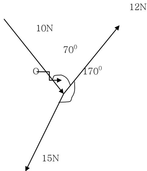
Figure shows a body of mass 5kg acted upon by forces of magnitudes 10N, 12N and 15N. Find the distance covered by body in 5 seconds.
