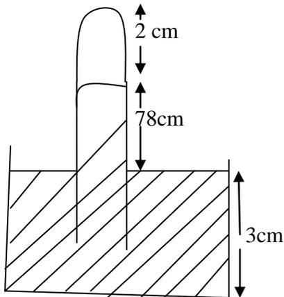
The diagram above in figure 5 shows a mercury barometer. Find the value of the atmospheric pressure
