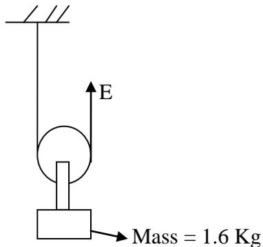
Figure 8 shows a light smooth pulley used to lift a mass of 1.6 kg by applying an effort E. The mechanical advantage of the system is
