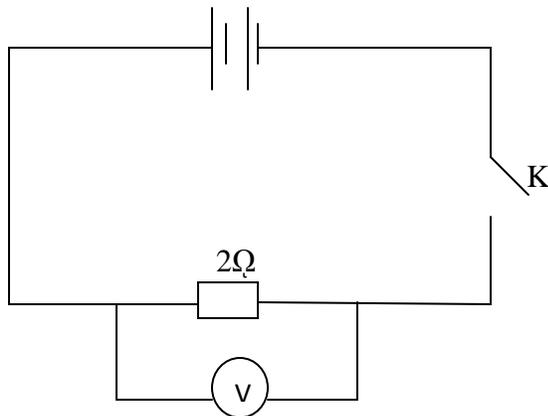
What will be the reading of the voltmeter when switch, K, is closed?
