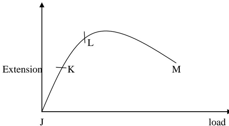
The diagram in figure 6 shows a graph that represents the extension of a wire with increasing load. At what region does the yield point occur?
