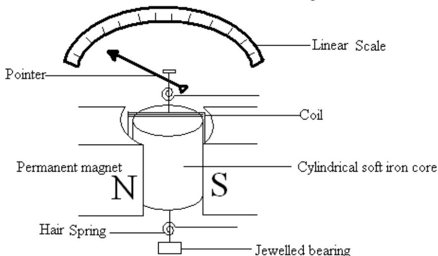
It consists of a rectangular coil with many insulated turns wound on an aluminum former, soft iron cylindrical core between the curved poles of a powerful permanent magnet, the springs which control the rotation of the coil, a pointer and a linear scale. The current is led in and out by two hair springs.
