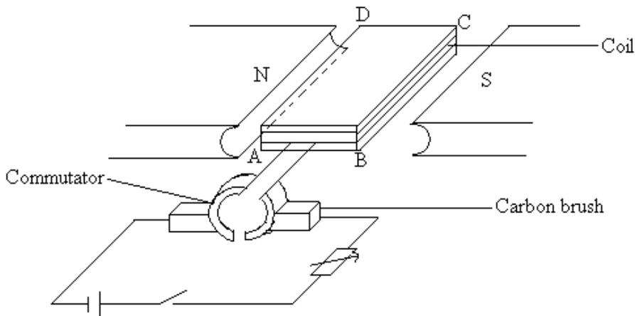
The d.c motor changes electrical energy to mechanical energy. It consists of a rectangular coil which can rotate about a fixed axis in a magnetic field provided by the permanent magnet. The ends of the coil are soldered to two halves of a copper ring (commutator), two carbon brushes press lightly against the commutators
