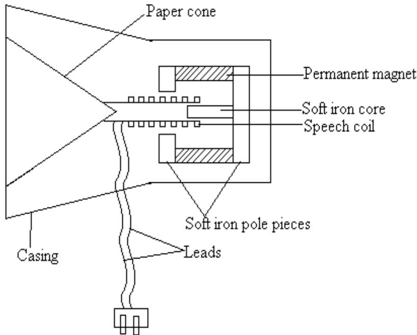
It consists of a light coil of wire known as a speech coil wound tightly round a cylindrical former to which a large thin cardboard cone is rapidly attached. The coil is in a radial magnetic field provided by the permanent magnet which has circular pole.
