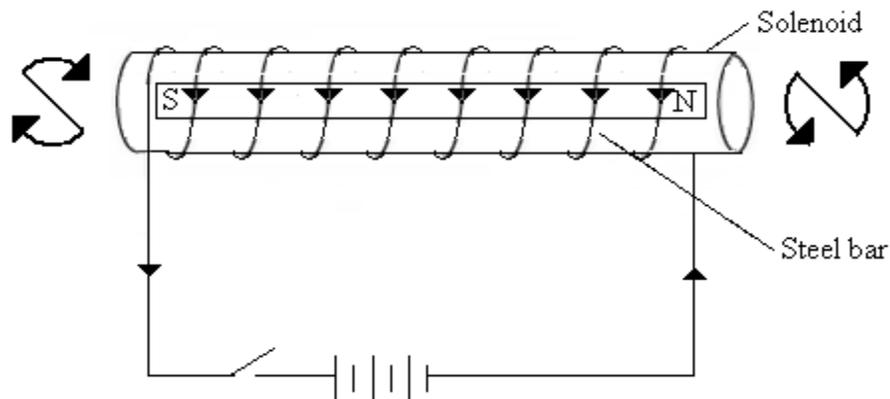
The material to be magnetized is inserted into a solenoid to which a steady d.c is flowing. The current is switched on for a short time. When the steel bar is removed, it is found to be magnetized. The current flowing in the same direction makes the atomic magnets in the Domains to point in the direction. The polarity of the steel bar depends on the direction in which the current is flowing.
