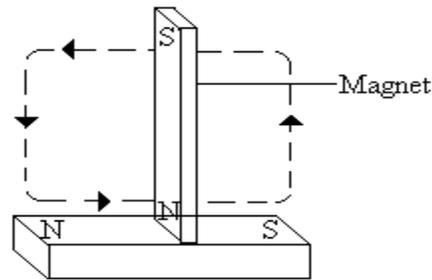
In this method, the steel bar is stroked from end to end several times in one direction with one pole of a magnet. The polarity produced at the end of the bar is of the opposite kind to that of the stroking pole.
