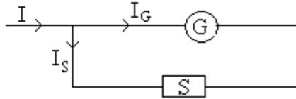
Most of the current will pass through the shunt and only a small part through the galvanometer.
