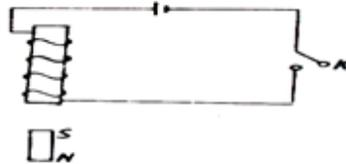
The diagram above shows a small magnet placed near an electromagnet. Describe what happens to it when the key K is closed. (02 marks)
