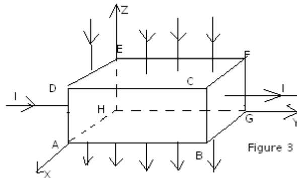
(c) Figure 3 shows a rectangular conductor ABCDEFGH carrying current I in a direction perpendicular to a vertical magnetic field of flux density B.
