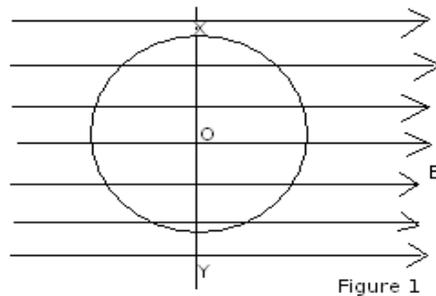
A circular loop of wire is placed in a uniform magnetic field of flux density  $B$ , with the axis of the wire as shown in figure 1. Explain what happens to the loop when current starts to flow through it in a clockwise direction if the loop is pivoted about the axis XOY. (3)
