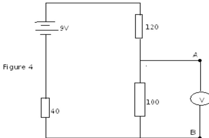
In the circuit in figure 4 the voltmeter V has resistance of  $400\Omega$
