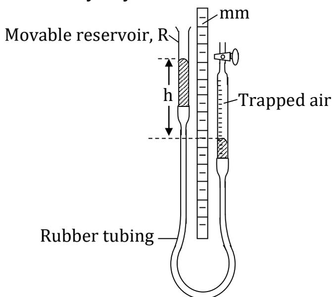
The apparatus consists of a graduated tube,  $T$ , connected by rubber tubing to a reservoir,  $R$ .
