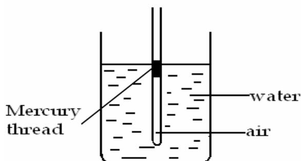
A graduated glass-tube containing air trapped below a mercury thread is immersed in a beaker of water and the water is heated as shown in the figure above.
