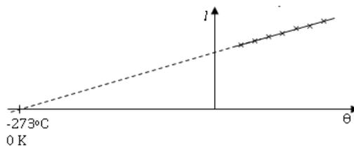
Now, throughout the experiment the pressure on the trapped air was constant, being atmospheric plus that due to the weight of the mercury in the tube.
