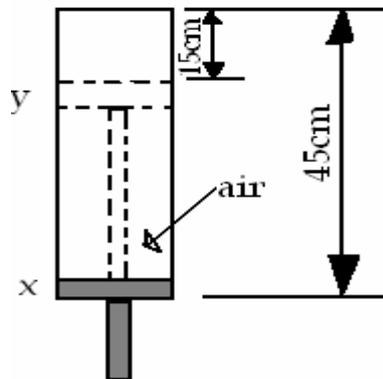
In figure above the piston is moved from X to Y at constant temperature. The air pressure is
