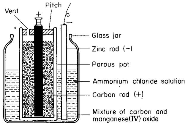
The leclanche wet cell is identical to the dry cell except that its electrolyte is liquid ammonium chloride solution.
