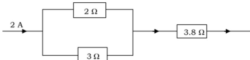
$$\text{Resistance in parallel } R_p = \frac{2 \times 3}{2+3} = \frac{6}{5} = 1.2 \Omega$$
