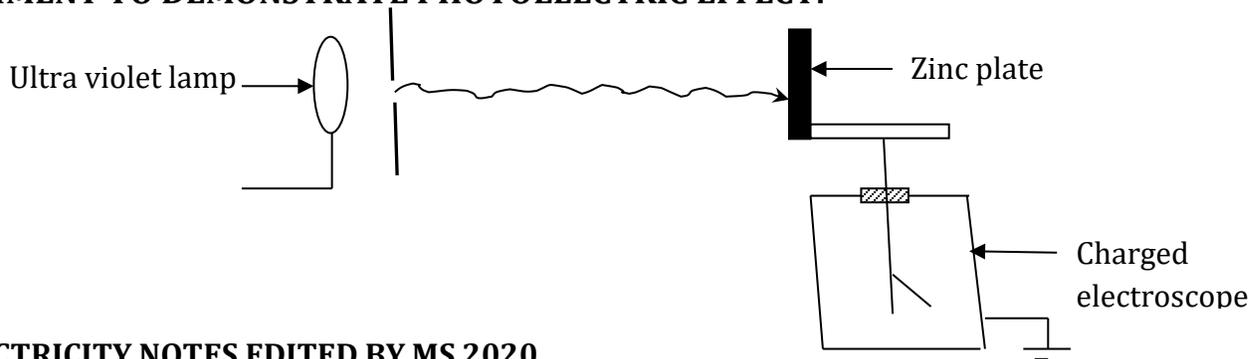
When Ultra violet light is incident on a clean zinc plate placed on the cap of a gold leaf electroscope:
