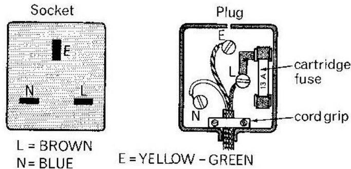
The fuse in the plug is connected to the live wire in the circuit.
