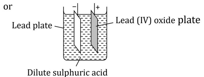
When fully charged, the relative density of the acid is 1.25 which falls to 1.18 at cell discharge.
