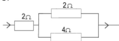
Resistance in parallel,  $R_p = \frac{R_1 R_2}{R_1 + R_2} = \frac{2 \times 4}{2 + 4} = \frac{8}{6} = \frac{4}{3}\Omega$ .
