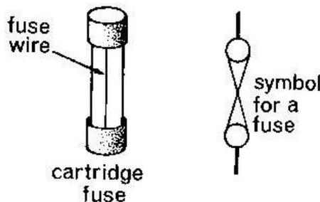
A fuse is a short length of a thin wire of low melting point which breaks the circuit when the current through it exceeds a safe value.
