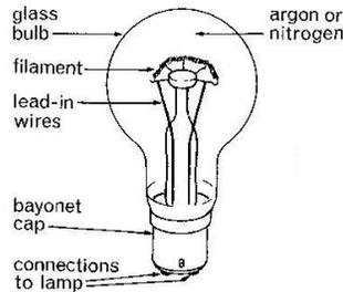
It consists of the filament made of a thin and coiled tungsten wire.
