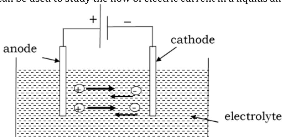
When an electric current passes through an electrolyte, a chemical reaction takes place at the surface of the electrodes. This process is known as **electrolysis**.
