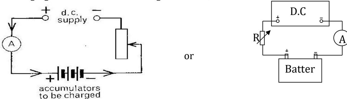
The supply must be d.c (direct current) of greater E.M.F than that of the accumulator.
