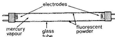
A Fluorescent tube has electrodes at fixed at both ends inside a partially evacuated glass tube whose inside walls are coated with a fluorescent powder and containing mercury vapour.
