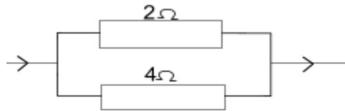
ANS: Effective resistance,  $R = \frac{R_1 R_2}{R_1 + R_2} = \frac{2 \times 4}{2 + 4} = \frac{8}{6} = \frac{4}{3} = 1.33\Omega$ .
