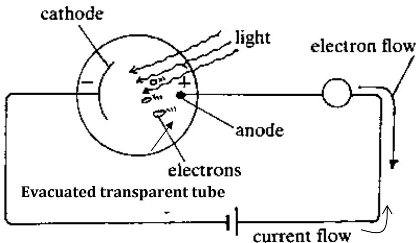
When a suitable radiation falls on the zinc cathode, it emits electrons by photoelectric emission. The anode attracts the electrons which then pass through an external circuit causing an electric current.
