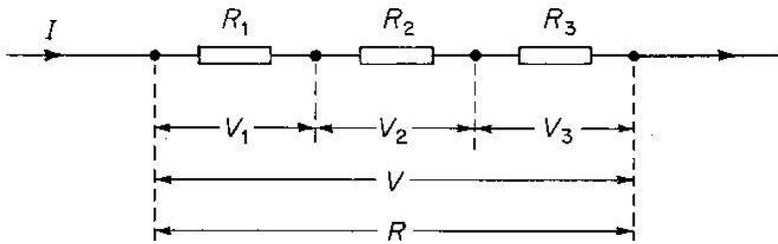
The same current,  $I$ , is passing through  $R_1, R_2$  and  $R_3$ .
