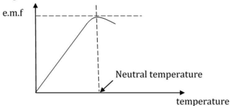
**Neutral temperature** is the temperature of the hot junction at which the e.m.f is a maximum. Thermocouples are used as small power supply in space satellites, weather buoys and weather ships.
