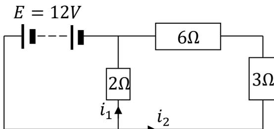
a battery of emf 12 V and negligible internal resistance is connected to resistances 2Ω, 3Ω, 6Ω as shown above find the currents  $I_1$  and  $I_2$ .
