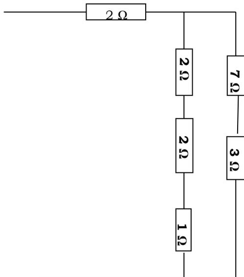
$$R_1 = R_7 + R_3 = 7 + 3 = 10\Omega \dots\dots\dots (1)$$
