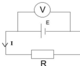
When the voltmeter is directly connected to the cell, it reads  $V = E$ , the e.m.f. of the cell.
